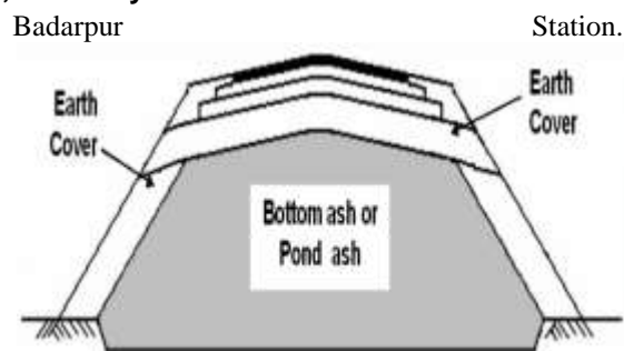
Fig.7. Road Embankment construction using fly ash.
