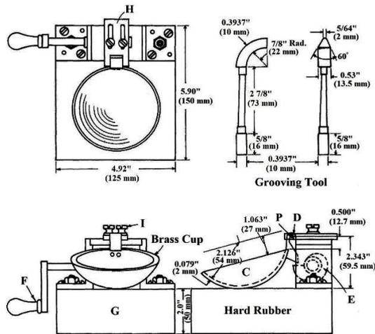
Fig. 3 Mechanical Liquid Limit Device [5].
