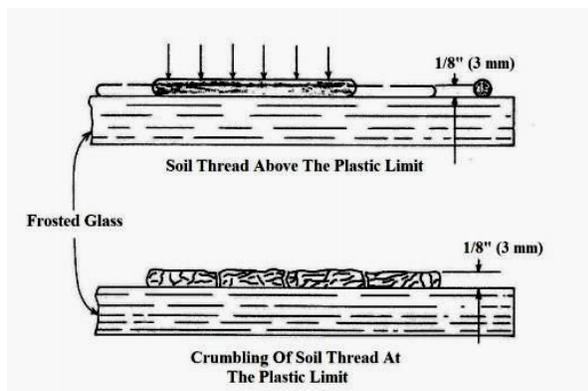
Fig.4 Plastic Limit Test [5]
