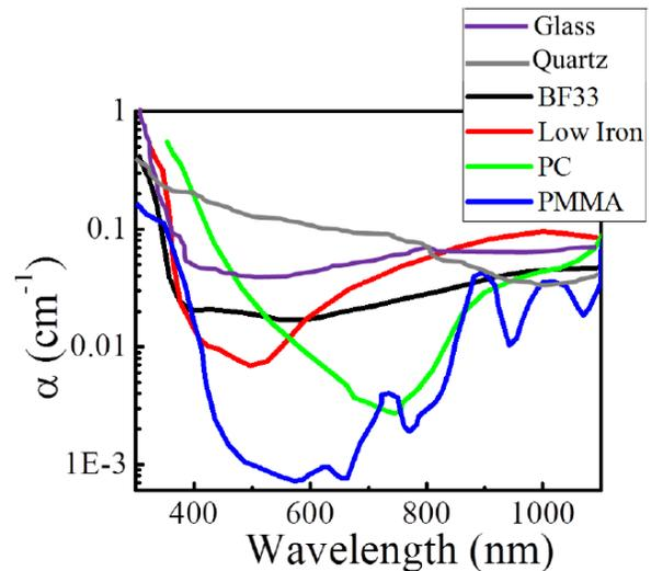
Fig. 2. Absorption coefficients of standard glass, quartz, BF33 glass, low iron glass, polycarbonate (PC) and poly(methyl methacrylate) (PMMA) as a function of wavelength<sup>[17]</sup>.
