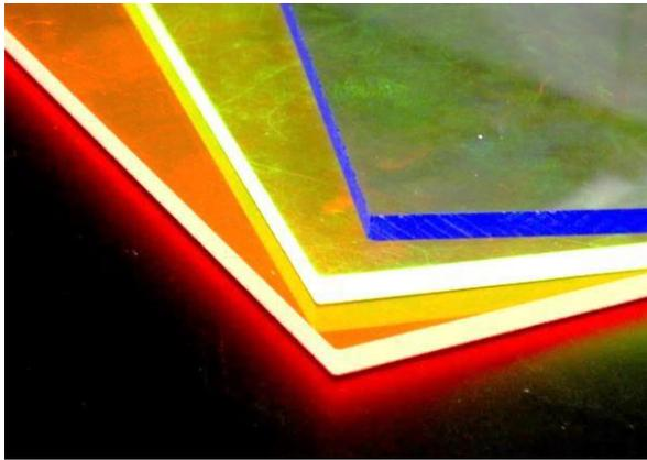
Fig. 1. Photograph of typical colorful luminescent solar concentrators highlighting the waveguided emission that is brightly focused at the edge.
