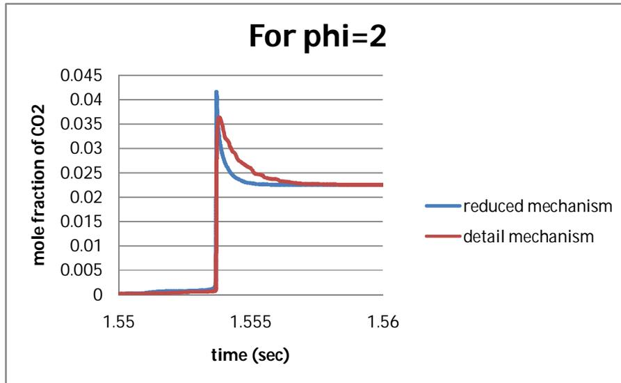
Fig. 3. Mole fraction of CO<sub>2</sub> for phi=2
