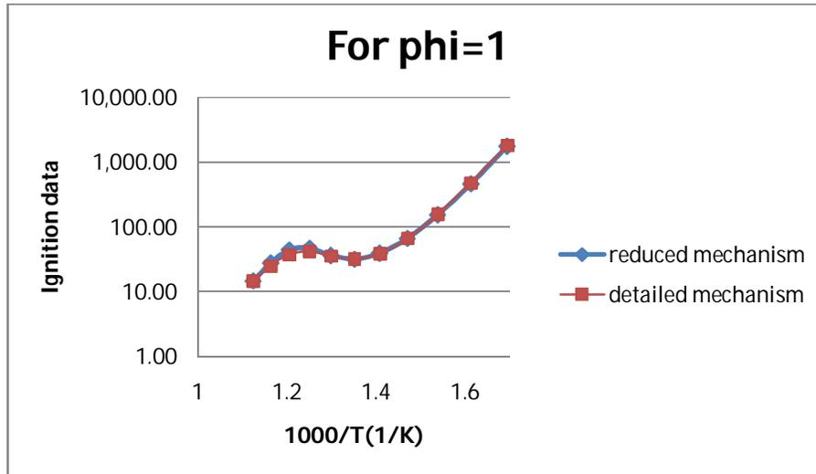
Fig. 1. Ignition data with NTC region for phi=1
