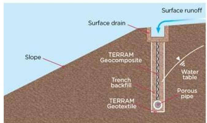
**Slopes and embankments.** The drainage function is a critical element in the design of soil slopes and in slip repairs.
