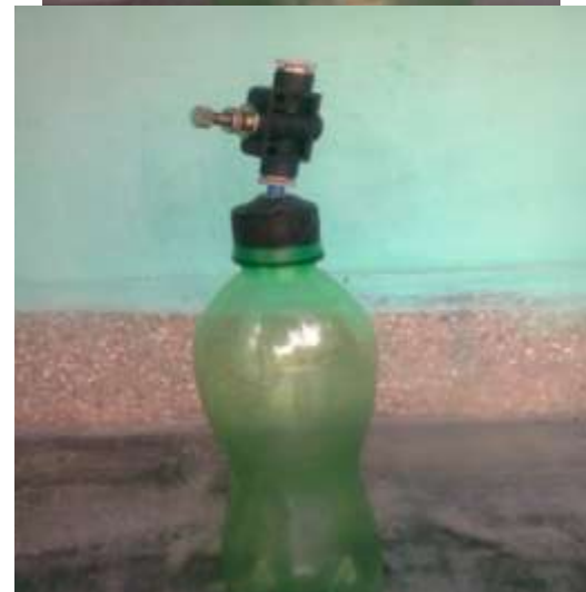
Figure 4: Storage Bottle for Compressed Biogas
