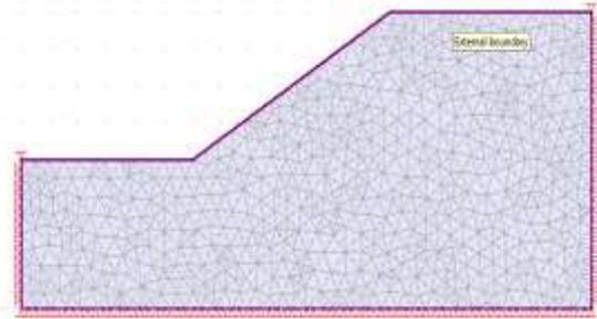
Fig. 1: Slope configuration-I ( at slope angle 30 deg)
