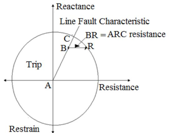
Fig. 3: Effect of fault resistance on reach of the impedance relay.
