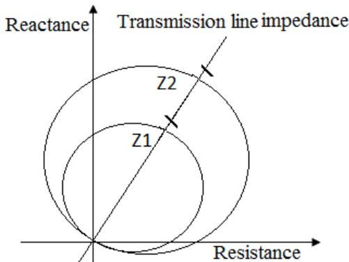
Fig. 1: Mho relay characteristics for two zones of protection.
