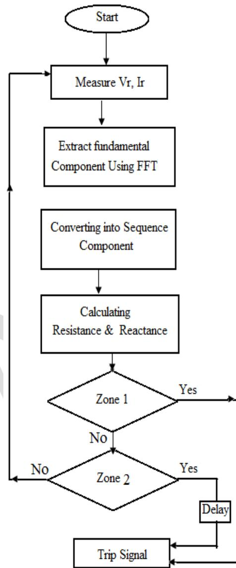
Fig. 5. Distance relay modeling Algorithm
