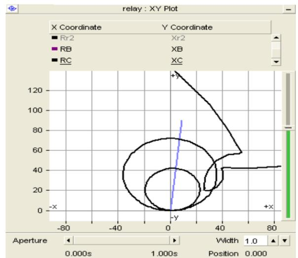
(b) Fault at 40 km with fault resistance 18Ω from Bus-A, Zone 1 of Mho Relay
