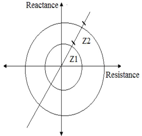
Fig. 2: Impedance relay characteristics for two zones of protection.
