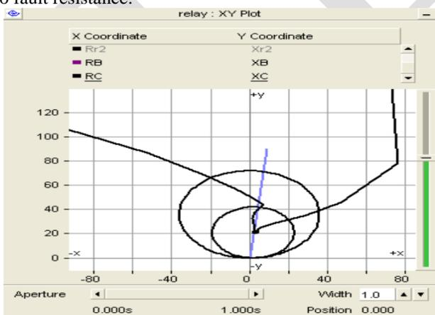
(a) Fault At 40 km with fault resistance 0.1Ohm from Bus-A, Zone 1 of Mho Relay
