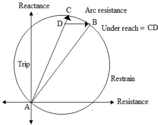
Fig. 4: Effect of fault resistance on reach of the mho relay.
