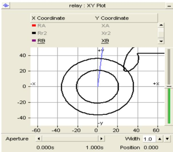
(b) Fault at 40km with Fault resistance of  $18\Omega$  from Bus-A, Zone 1 of Impedance Relay
