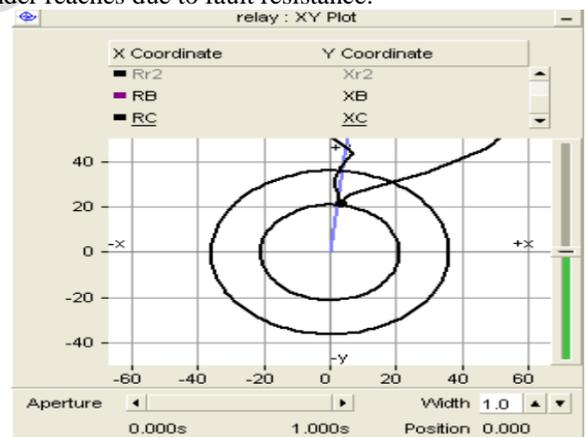
(a) Fault at 40km with Fault resistance of 0.1Ω from Bus-A, Zone I of Impedance Relay
