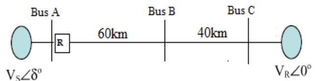
Fig. 6. Single line diagram of Transmission line.
